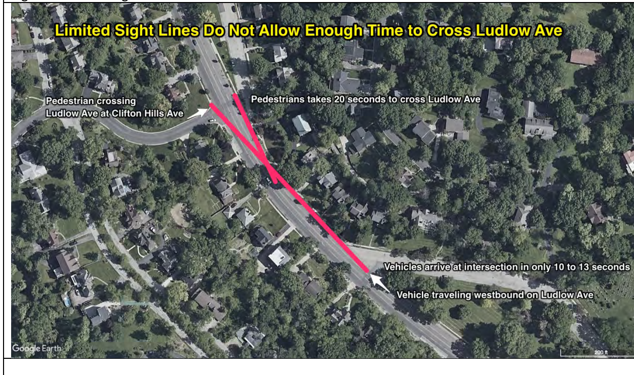
Figure 7 Limited Sight Lines at Clifton Hills Ave and Ludlow Ave
